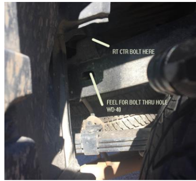
Figure 6 Right Center Bolt Lube Location
