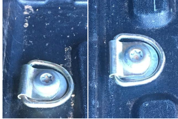
Figure 2 Mounted Front Left & Center Left (V-Ring Same)
