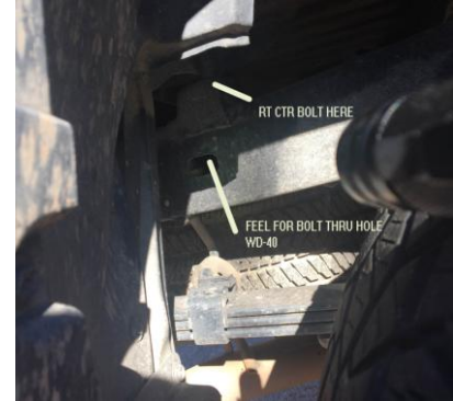
Figure 3 Right Center Bolt Lube Location
