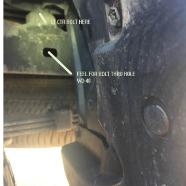
Figure 2 Left Center Bolt Lube Location
